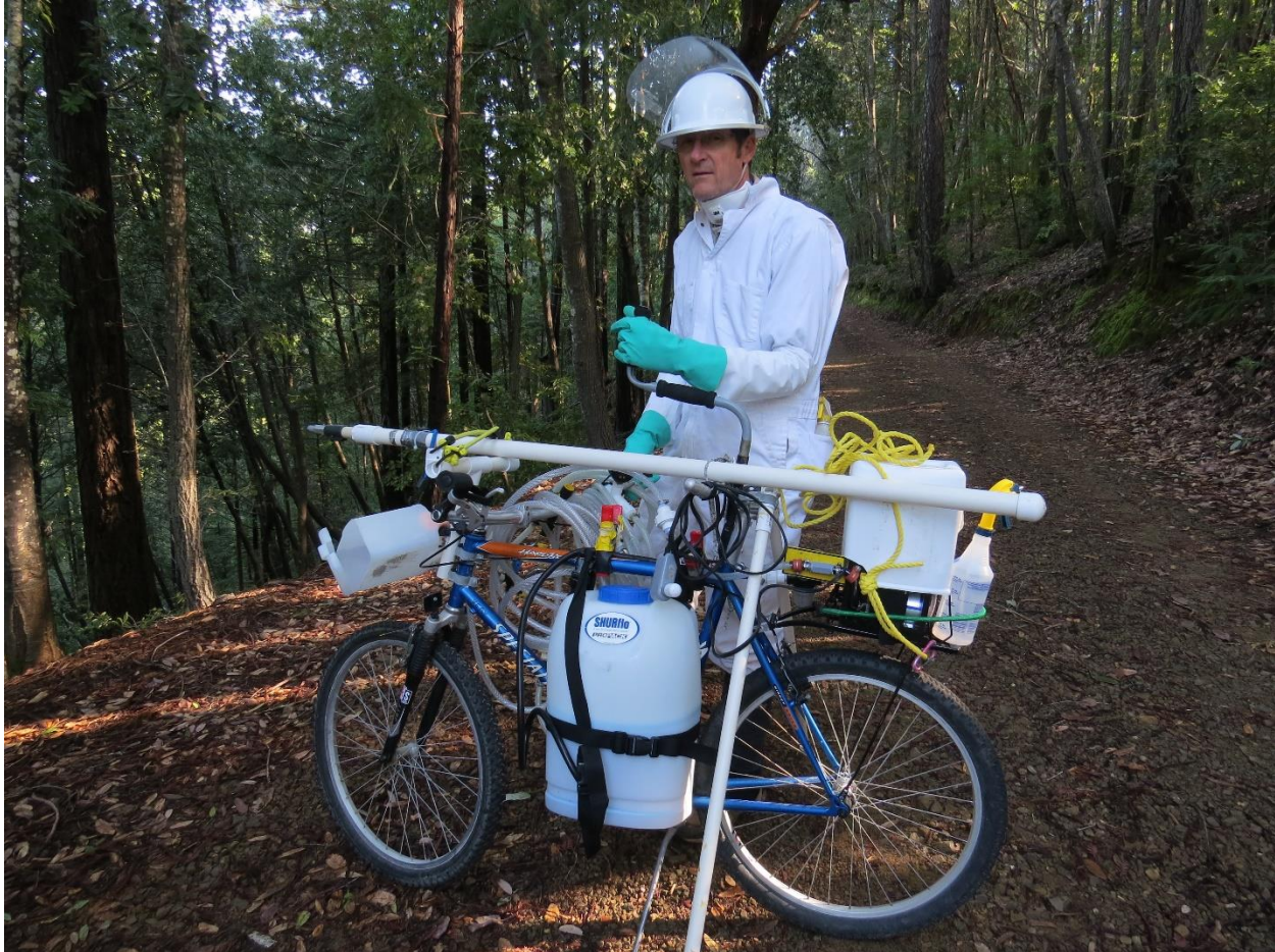
Figure 1-3. The bicycle-mounted sprayer uses a 12 VDC pump/speed controller/battery assembly mounted on the back rack (under white housing) that is activated by an electric switch (gray electric box at end of black cord by top of tank). The telescoping spray pole, hoses and other components are attached to racks and other points on the bicycle for transport. A rope was attached at the front or back to allow a second person to belay or assist in pulling the bike on steep terrain.
