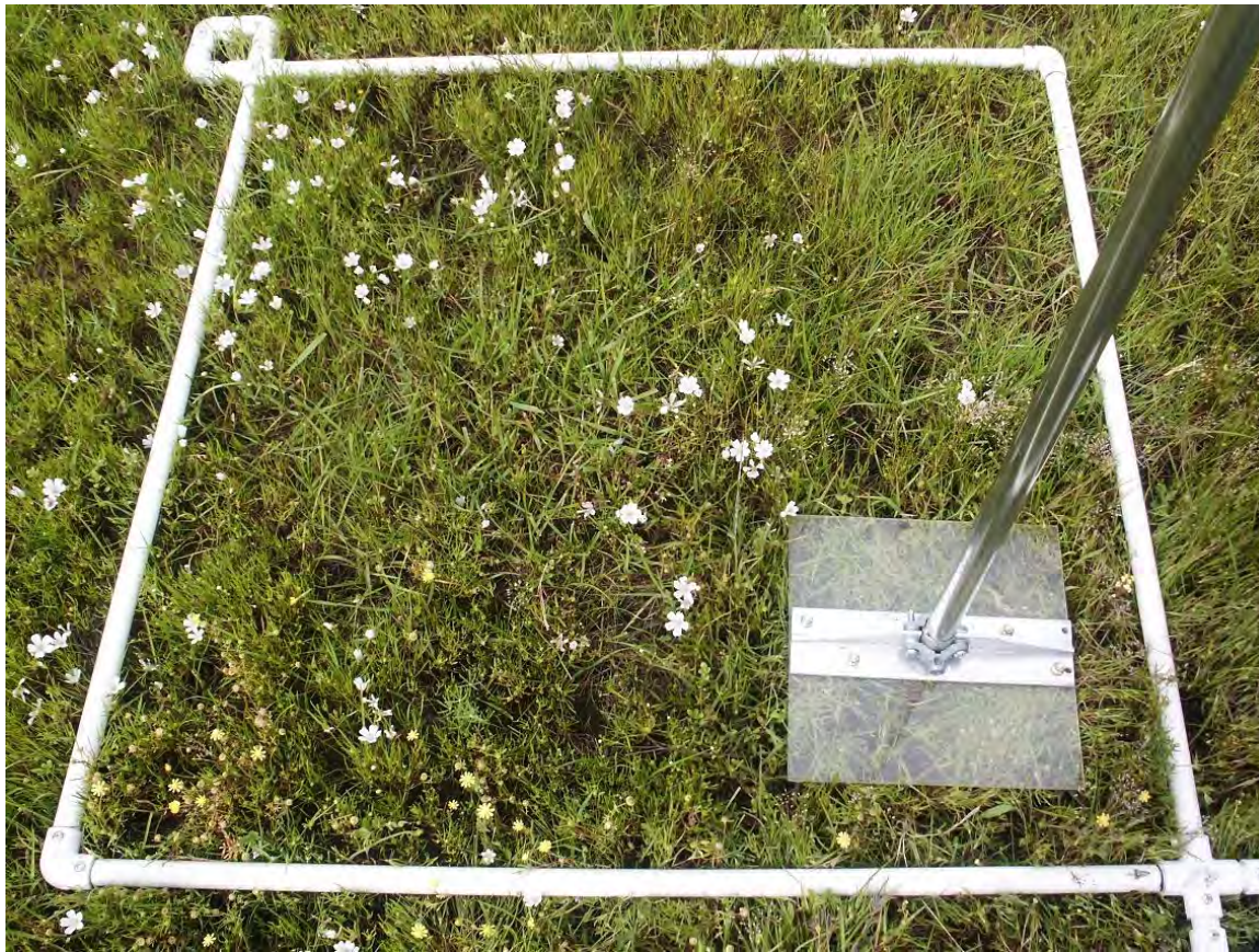
Figure 2. Falling plate meter in grazed plot.
