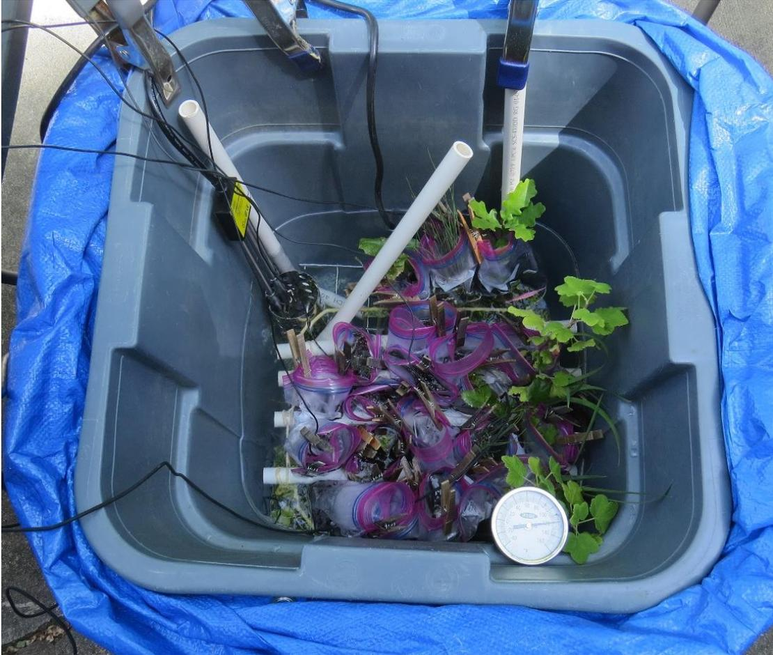
Figure 2. Water bath setup for tests 4A and B. PVC pipes were used to keep containers submerged. Bucket heater is at upper left. Wires are for dataloggers measuring temperatures and the thermostat.
